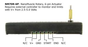
N/C: Not Connected START: HIGH (V+) when actuator is at rest END: HIGH (V+) when actuator is at end of stroke Note: No safe capability: do not over heat SMA wires
