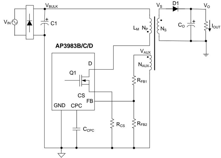
Figure 1. Simplified Flyback Converter Controlled by AP3983B/C/D
