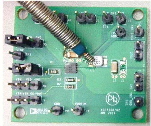
Figure 2. Output Ripple Measurement
