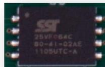
See the [SST25VF064C data sheet](#) for hardware specifications and programming details and the Renesas SH7269 datasheet for information on the SPI master port configuration. **PF2** is a generic I/O pin on the SH7269 and is wired (with a weak pull-up) to the FLASH's **RESET#** input. Left unprogrammed, the FLASH will self-reset on power-up and be in
