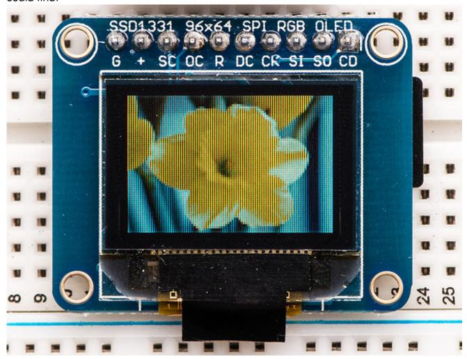
This OLED uses the SSD1331 driver chip, which manages the display. You can talk to the driver chip using either 3 or 4-wire write-only SPI (clock, data, chip select, data/command and an optional reset pin) or standard 8-bit parallel 8080/6800 which also permits reading pixel data from the display. Our example code shows how to use SPI since for such a
