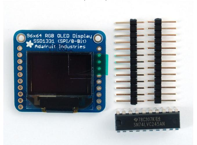
Since the OLED is 3.3V and also uses 3.3V logic, we need to use a logic shifter. We include a DIP logic shifter, the 74LVX245 with the OLED. If you're using a 3.3V logic chip, you can skip the logic shifter. Arduinos are all 5.0V so we'll be demonstrating that.
