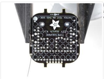
Bend the wire leads out so the resistor sits flat against the PCB. Then you can flip it over and it wont fall out!
