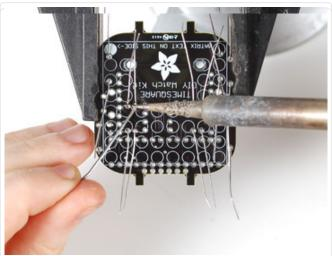
Solder in all the resistors, either one at a time or all 8 at once! Make sure you don't forget any solder points, though.
