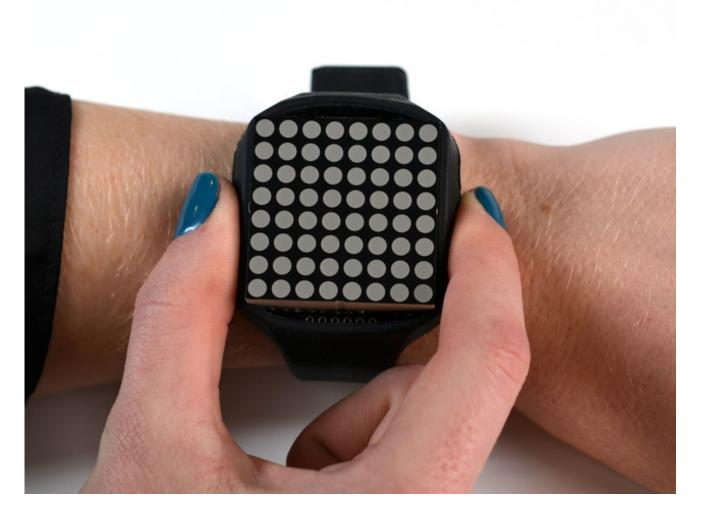
First wake the watch by **tapping** either side button. With the time display active, you can enter time-setting mode by **holding** down **both** side buttons for about two seconds. If using the watch for the first time, or after swapping batteries, it may wake in time-setting mode automatically.
