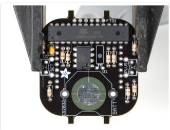
Next we'll do the big microcontroller chip. This chip is the brains, it does all of the displaying and button handling. Most of the time its 'sleeping' and when you press a button it wakes up and shows the time. It has a lot of pins because the matrix requires 16 pins to draw, and then you need some more pins for buttons, the RTC chip, reprogramming, etc.
