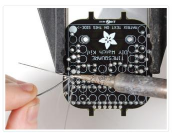
You did great with the first two parts, now we will solder in the remaining resistors **R1-R8**. These resistors are the LED 'choke' resistors - they keep the LED matrix's light even and avoids having too much current draw that would kill the battery off!
