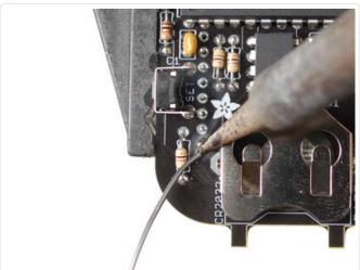
Now solder in all the pins of the matrix, you may have to angle the iron tip a bit to avoid burning other parts
