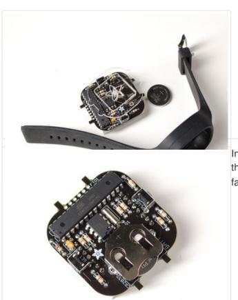
Insert a 20mm (CR2032) coin cell battery so that the flat + side is facing up and the bumpy side is facing down into the PCB
