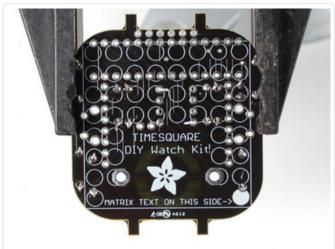
The important thing about chips is that they are not like resistors and capacitors in that they **can't** be placed 'either way'. It **must** be placed the right way or the chip wont work. Look for the end of the chip with a notch and a dot. These must match up the silkscreened image on the PCB so make sure the notches line up.
