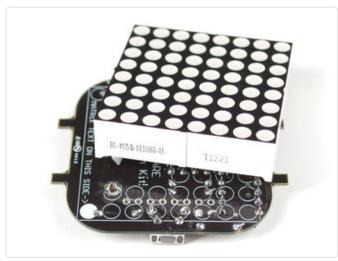
side must go on the side of the PCB with a dot as you see here. Also the matrix goes on the OPPOSITE side of the other parts!
