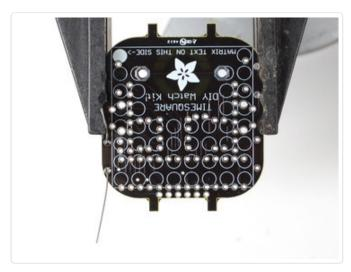
Once the soldering is complete, we can clean up by clipping the leads of the resistor. This keeps them
