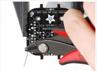
from shorting to something else. Use diagonal or flush cutters to clip the wires right above where the solder joint ends.
