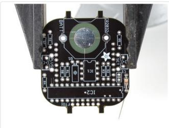
Start by placing the PCB in a vise to keep it steady. We'll be soldering parts on TOP, where the silkscreen shows the component placing. The first part we'll place is the 10K resistor. This resistor is marked **brown black orange gold**. (It's also the only single resistor of that color)
