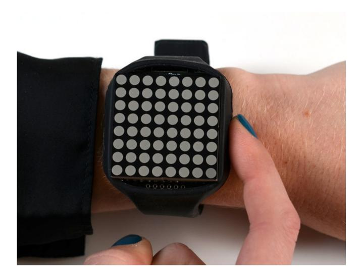
There are two digits each for the year, month, day, hour and minute, and the watch will briefly display the symbols **Y**, **M**, **D**, etc. when moving from one pair of digits to the next. The high and low digits are set individually...this is different from most digital clocks, we find it faster and less troublesome. The range for each digit varies, and the watch will keep the values in check.
