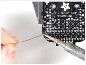
With your soldering iron heated up and ready, solder in both leads of the resistor. To do this, heat up the round ring pad and the wire lead at the same time for 2 or 3 seconds, then dip the end of the solder into the heated joint to melt it in.
