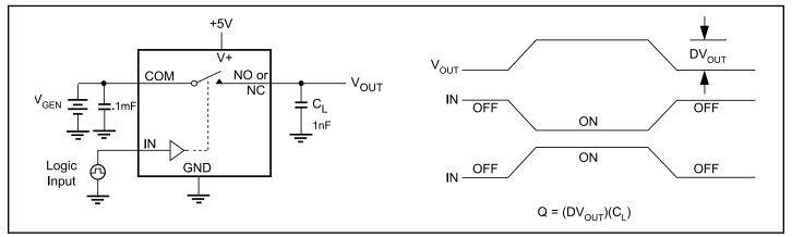
Figure 2. Charge Injection
