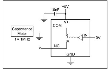
Figure 6. Channel-On Capacitance
