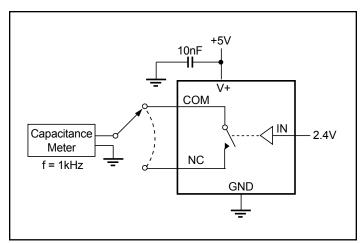
Figure 5. Channel-Off Capacitance
