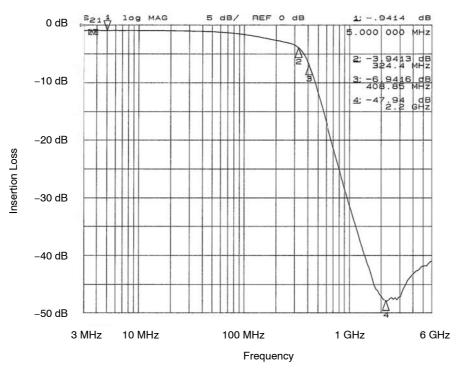
Figure 5. Filter 1 Insertion Loss (CM1461-06DE)
