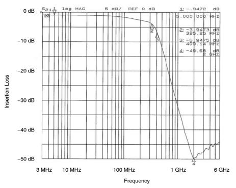
Figure 9. Filter 5 Insertion Loss (CM1461-06DE)
