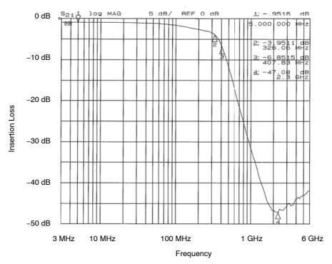
Figure 8. Filter 4 Insertion Loss (CM1461-06DE)
