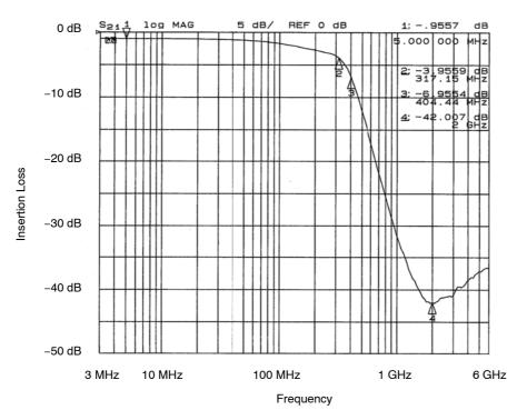
Figure 11. Filter 1 Insertion Loss (CM1461-08DE)
