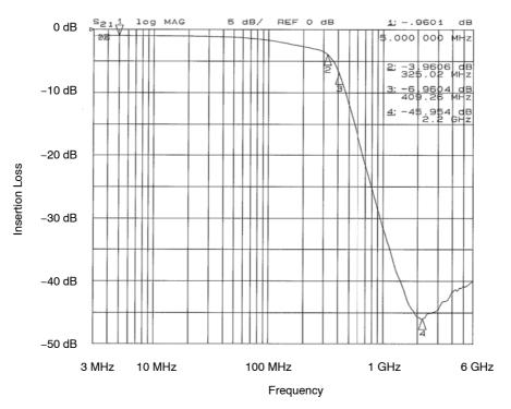
Figure 7. Filter 3 Insertion Loss (CM1461-06DE)
