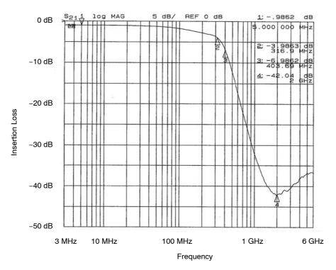
Figure 4. Filter 4 Insertion Loss (CM1461–04DE)
