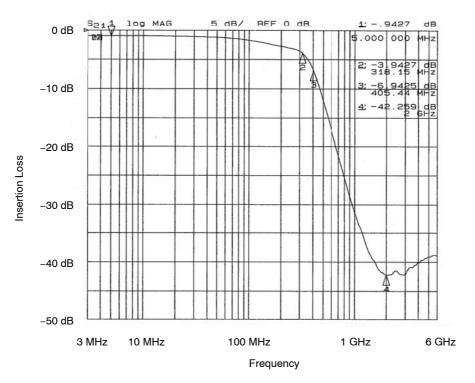
Figure 3. Filter 3 Insertion Loss (CM1461-04DE)
