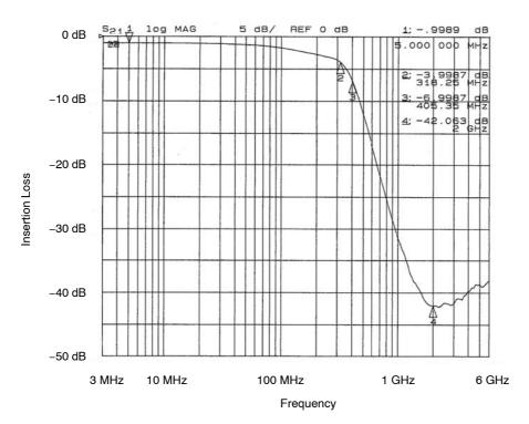
Figure 2. Filter 2 Insertion Loss (CM1461-04DE)
