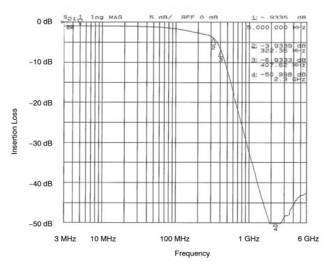
Figure 10. Filter 6 Insertion Loss (CM1461-06DE)
