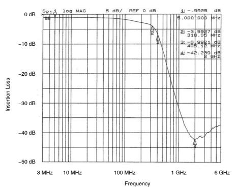
Figure 1. Filter 1 Insertion Loss (CM1461-04DE)
