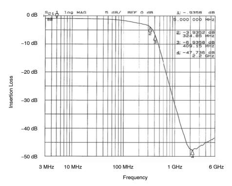
Figure 6. Filter 2 Insertion Loss (CM1461-06DE)
