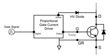
Figure 29: Simplified Voltage Controlled Proportional Driver
