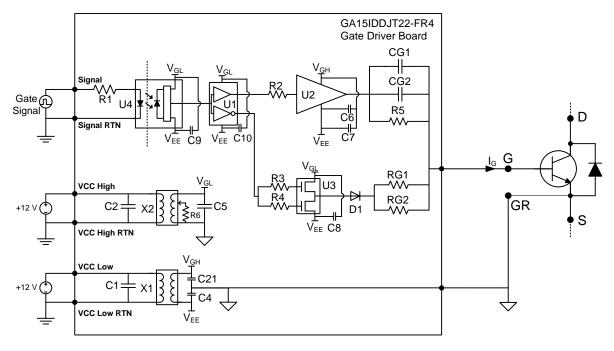
Figure 25: Topology of the GA15IDDJT22-FR4 Two Voltage Source gate driver.
