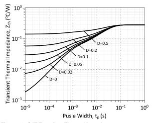
Figure 20: SJT Transient Thermal Impedance
