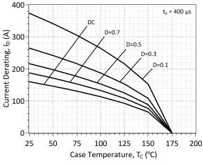
Figure 17: Drain Current Derating vs. Temperature
