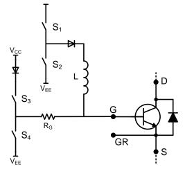
Figure 28: Simplified Inductive Pulsed Drive Topology
