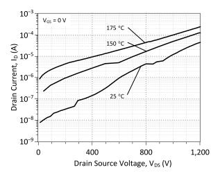
Figure 8: Typical Blocking Characteristics
