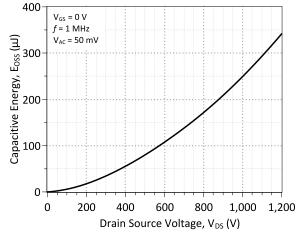
Figure 10: Energy Stored in Output Capacitance
