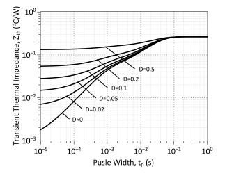
Figure 21: FWD Transient Thermal Impedance
