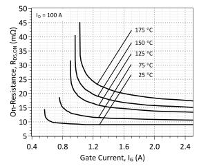
Figure 5: On-Resistance vs. Gate Current
