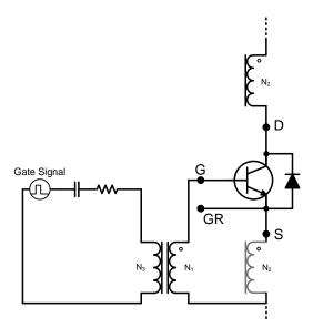
Figure 30: Simplified Current Controlled Proportional Driver
