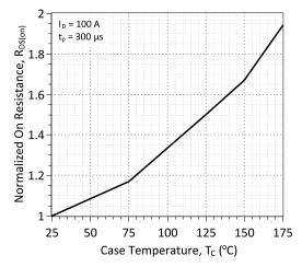
Figure 6: Normalized On-Resistance vs. Temperature
