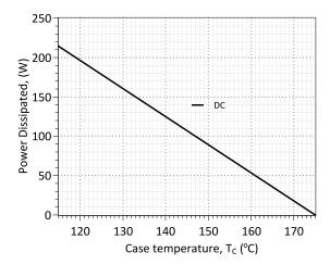
Figure 16: Power Derating Curve
