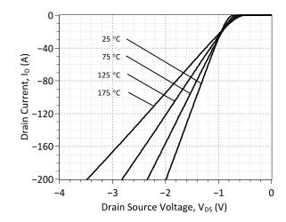
Figure 22: Typical FWD Forward Characteristics
