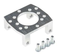
**Description:** The E Style Motor mount connects to the inside of Actobotics channels and works with both standard and precision gear motors. This allows you to drive shafts through channels. The mount utilizes various hole patterns for your motor, and a 1.5" hole pattern for connecting to other Actobotics products. The E Style mount is made from resilient 6061-T6 aluminum and weighs only 0.35oz.
