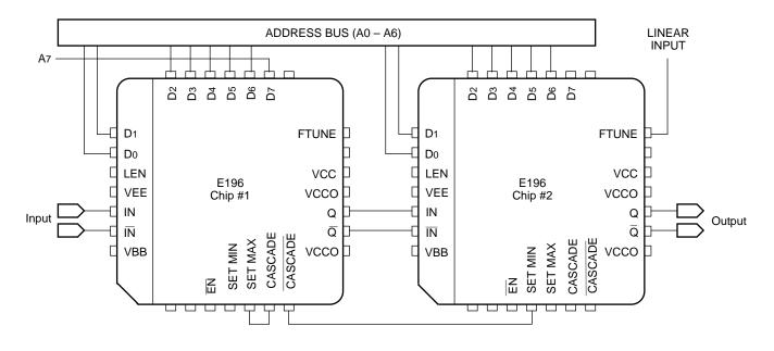
Figure 1. Cascading Interconnect Architecture
