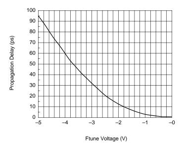
Propagation Delay vs Ftune Voltage (10E196)
