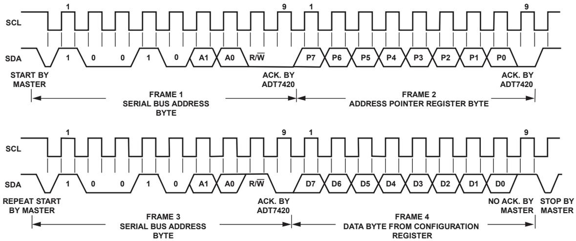
Figure 16. Reading Back Data from the Configuration Register
