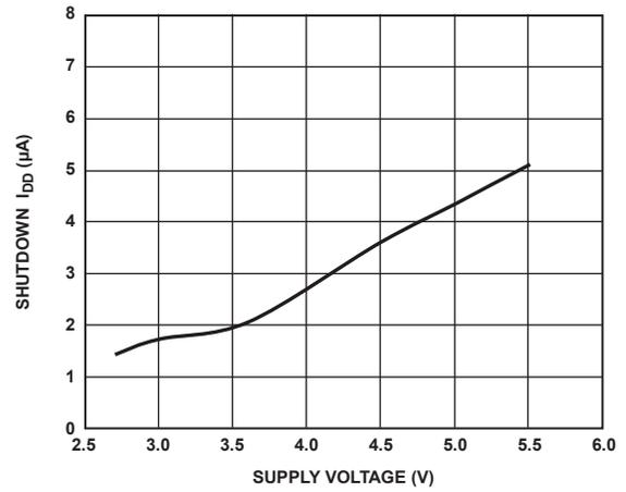
Figure 9. Shutdown Current vs. Supply Voltage
