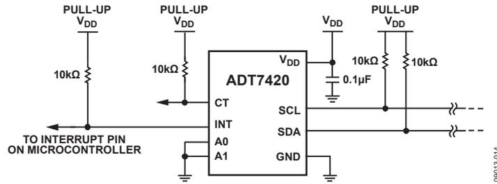
Figure 13. Typical I<sup>2</sup>C Interface Connection
