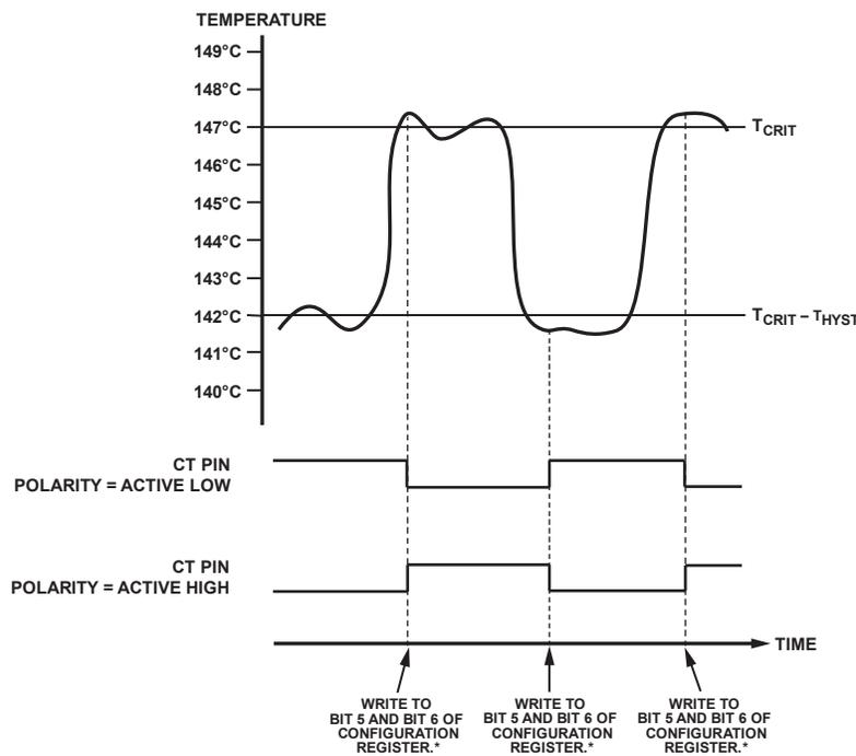
\*THERE IS A 240ms DELAY BETWEEN WRITING TO THE CONFIGURATION REGISTER TO START A STANDARD ONE-SHOT CONVERSION AND THE CT PIN GOING ACTIVE. THIS IS DUE TO THE CONVERSION TIME. THE DELAY IS 60ms IN THE CASE OF A ONE-SHOT CONVERSION.
