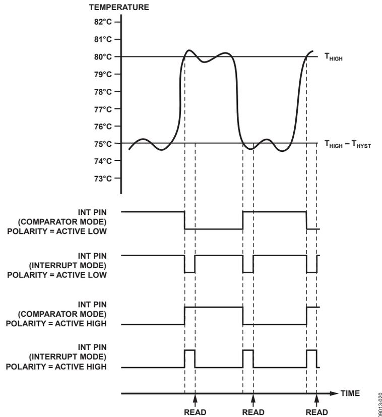
Figure 18. INT Output Temperature Response Diagram for T<sub>HIGH</sub> Overtemperature Events
