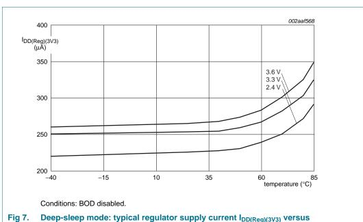
Fig 7. Deep-sleep mode: typical regulator supply current I<sub>DD(Reg)(3V3)</sub> versus temperature
