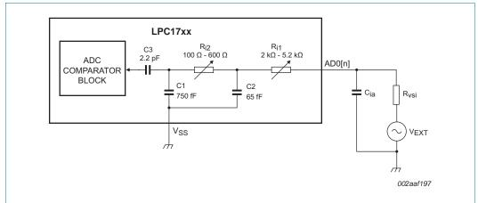
The values of resistor components  $R_{i1}$  and  $R_{i2}$  vary with temperature and input voltage and are process-dependent (see Table 20).
