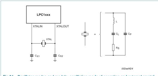
Fig 34. Oscillator modes and models: oscillation mode of operation and external crystal model used for  $C_{X1}/C_{X2}$  evaluation
