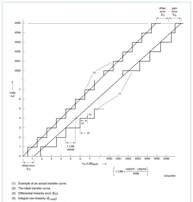
(5) Center of a step of the actual transfer curve.
