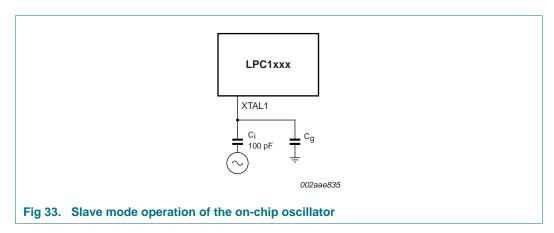
In slave mode the input clock signal should be coupled by means of a capacitor of 100 pF (Figure 33), with an amplitude between 200 mV(RMS) and 1000 mV(RMS). This corresponds to a square wave signal with a signal swing of between 280 mV and 1.4 V. The XTALOUT pin in this configuration can be left unconnected.
