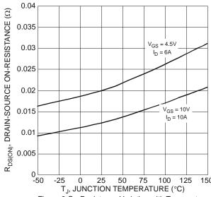
Figure 6 On-Resistance Variation with Temperature
