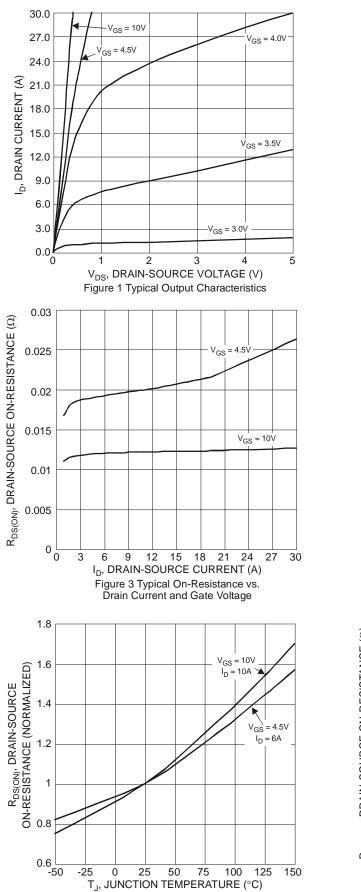
Figure 5 On-Resistance Variation with Temperature
