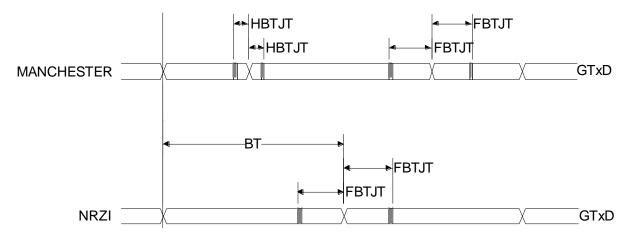
Figure 12. GSC Transmit Timings (Internal Baud Rate Generator)
