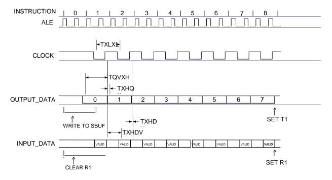
Figure 10. Shift Register Mode Timing Waveforms
