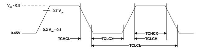
Figure 9. External Clock Drive Waveform
