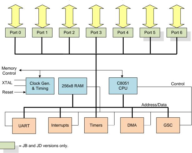
I/O for Memory, GSC, DMA, UART, Interrupts, and Timers
