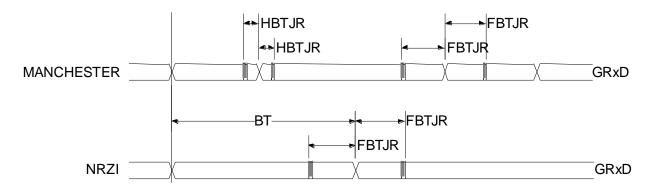
Figure 11. GSC Receiver Timings (Internal Baud Rate Generator)
