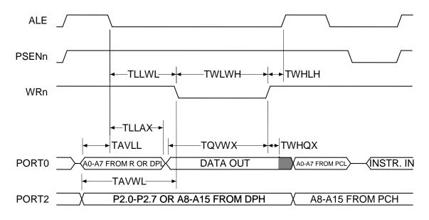
Figure 8. External Data Memory Write Cycle
