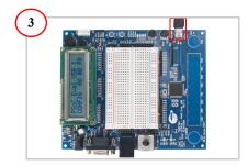
Connect the USB cable. LED5 lights up. The message "PSoC Eval USB 1" is displayed on the LCD. Observe that the mouse pointer on the PC screen moves in a square fashion.
