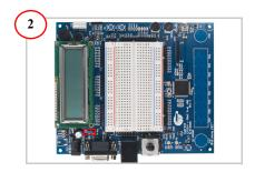
Ensure that P3, the power selection jumper (shunt), is placed on the first two pins (designated as VBUS).
