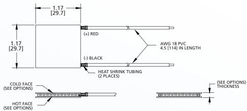
Ceramic Material: Alumina (Al<sub>2</sub>O<sub>3</sub>) Solder Construction: 138°C, Bismuth Tin (BiSn)
