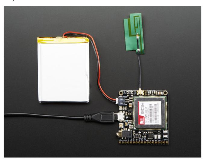
Then press the small **KEY** button next to the battery & cell antenna for 5 seconds. Then the computer will recognize a multi-type USB connection. <u>Install the drivers</u> (http://adafru.it/jFn)
