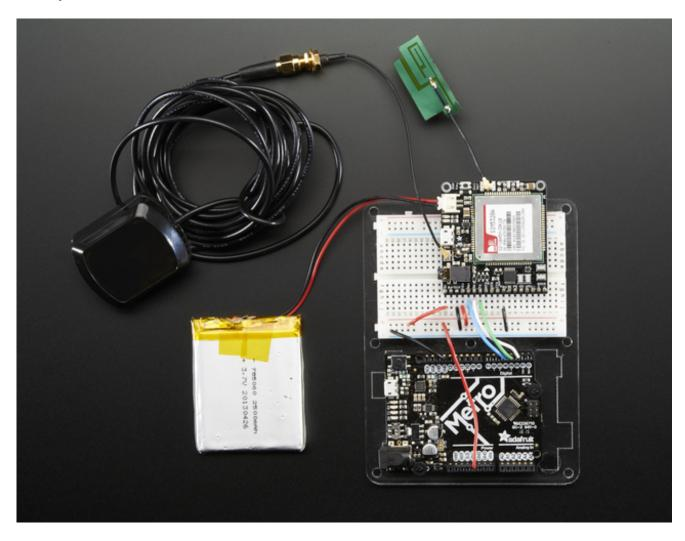
Check polarity for the battery!
