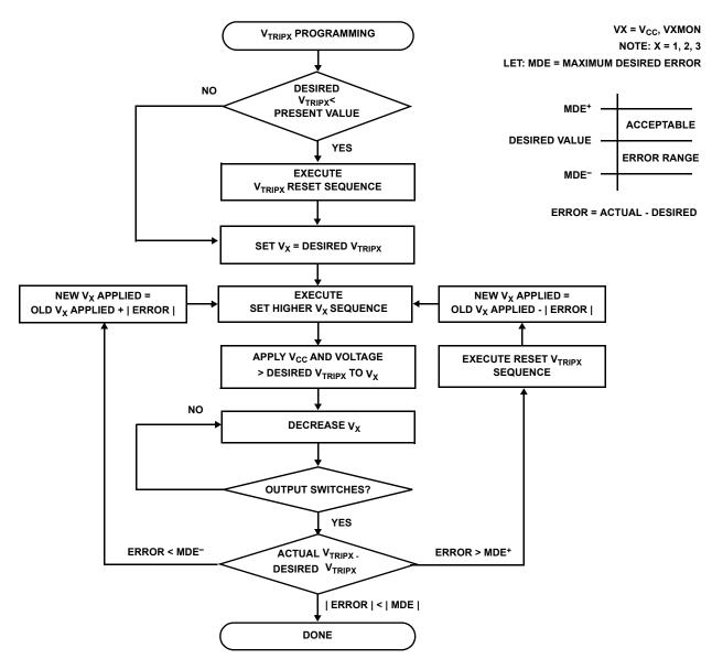
FIGURE 6. V<sub>TRIPX</sub> SET/RESET SEQUENCE (X = 1, 2, 3)
