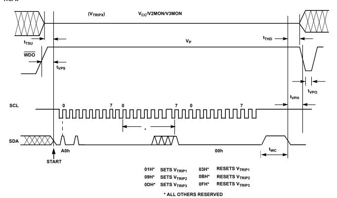
VTRIP1, VTRIP2, VTRIP3 Programming Specifications V<sub>CC</sub> = 2.0V to 5.5V; Temperature = +25°C
