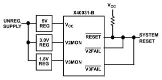
NOTICE: NO EXTERNAL COMPONENTS REQUIRED TO MONITOR THREE VOLTAGES.
