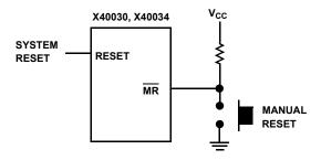
FIGURE 1. CONNECTING A MANUAL RESET PUSH-BUTTON
