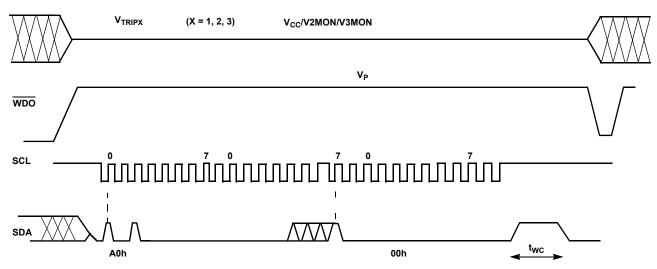
FIGURE 3. V<sub>TRIPX</sub> SET/RESET CONDITIONS
