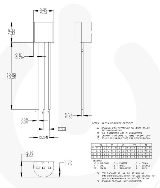
Figure 10. 3-LEAD, TO92, JEDEC TO-92 COMPLIANT STRAIGHT LEAD CONFIGURATION (OLD TO92AM3) (ACTIVE)
