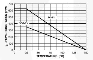
Figure 9. Power Dissipation vs. Ambient Temperature
