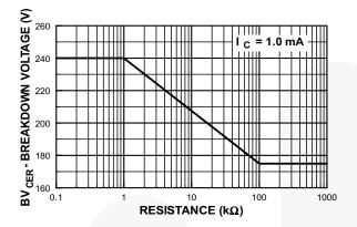
Figure 7. Collector- Emitter Breakdown Voltage with Resistance between Emitter-Base
