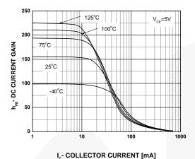
Figure 1. Typical Pulsed Current Gain vs. Collector Current
