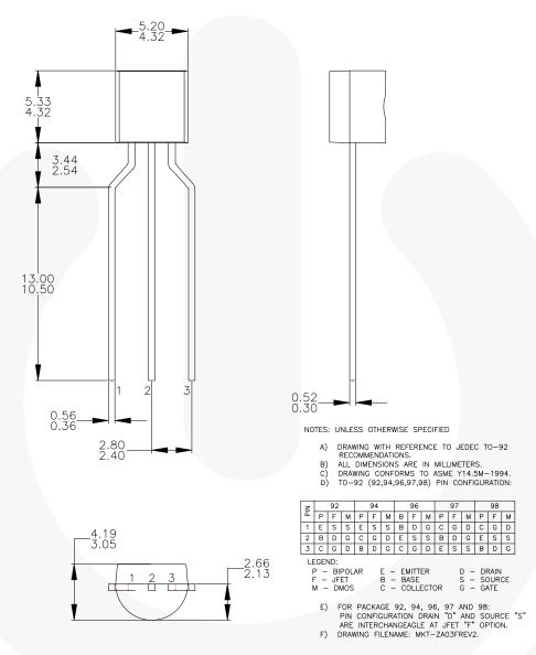
Figure 11. 3-LEAD, TO92, MOLDED, 0.200 IN-LINE SPACING LD FORM(J62Z OPTION) (ACTIVE)
