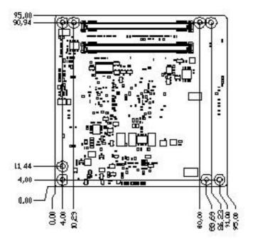
Figure 2.4 Board Dimension (Solder side)
