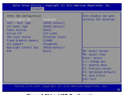
Figure 3.20 Intel IGD Configuration
