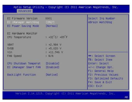
Figure 3.11 Embedded Controller Configuration
