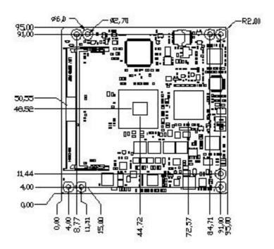
Figure 2.3 Board Dimension (Component side)
