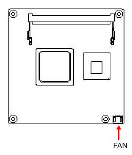
Figure 2.1 Board Layout (component side)
