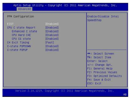
Figure 3.17 PPM Configuration
