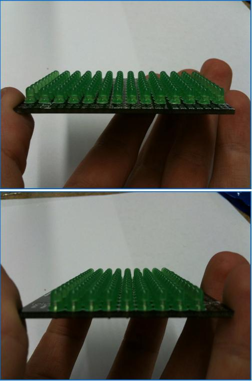
By looking down the rows and columns, you can see which LEDs are straight or crooked. This is much easier to fix when only one lead is soldered in, and it's easiest to find them along the way. Straightening them all at the end is quite a bit more difficult.
