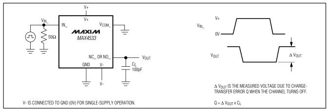
Figure 4. Charge Injection
