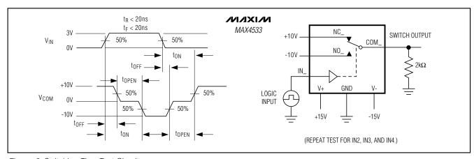
Figure 2. Switching-Time Test Circuit
