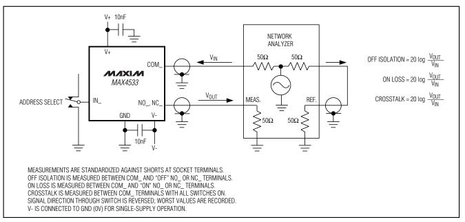
Figure 6. Frequency Response, Off-Isolation, and Crosstalk
