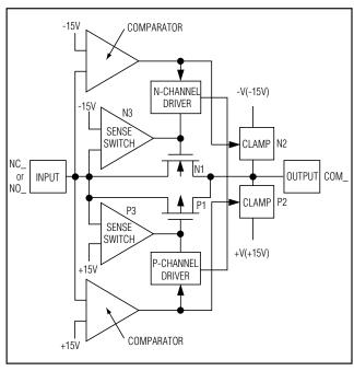
Figure 1. Simplified Internal Structure
