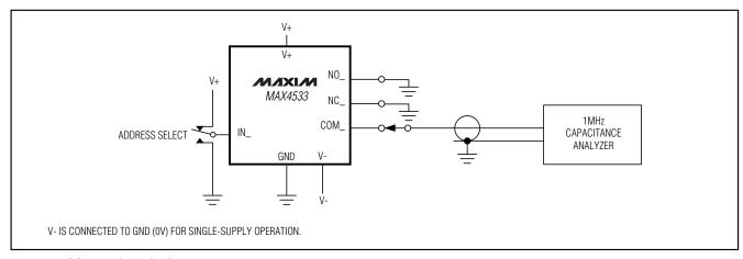
Figure 5. COM\_, NO\_, NC\_ Capacitance
