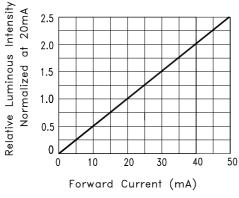
Fig.4 Relative Luminous Intensity vs. Forward Current
