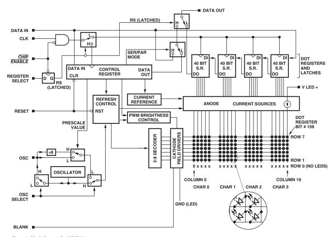
Figure 6. Block diagram for HCMS-39xx
