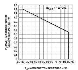
Figure 9. Maximum power dissipation per IC versus ambient temperature
