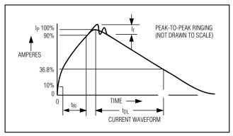
Figure 3. Human Body Model Current Waveform
