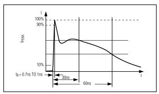
Figure 5. IEC 1000-4-2 Generator Current Waveform
