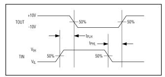
Figure 1. Transmitter Propagation-Delay Timing
