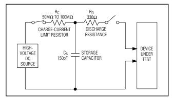
Figure 4. IEC 1000-4-2 ESD Test Model
