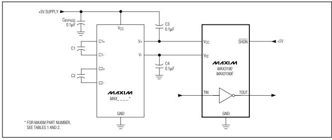
Figure 6. Powering the MAX3190/MAX3190E
