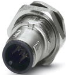
Sensor/actuator flush-type connector, 5-pos., M12 SPEEDCON, A-coded, rear/screw mounting with Pg9 thread, with straight solder connection
