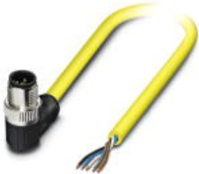
Sensor/Actuator cable, 5-position, TPE, yellow RAL 1021, Plug angled M12 SPEEDCON, A-coded, on free cable end, Cable length: 10 m
