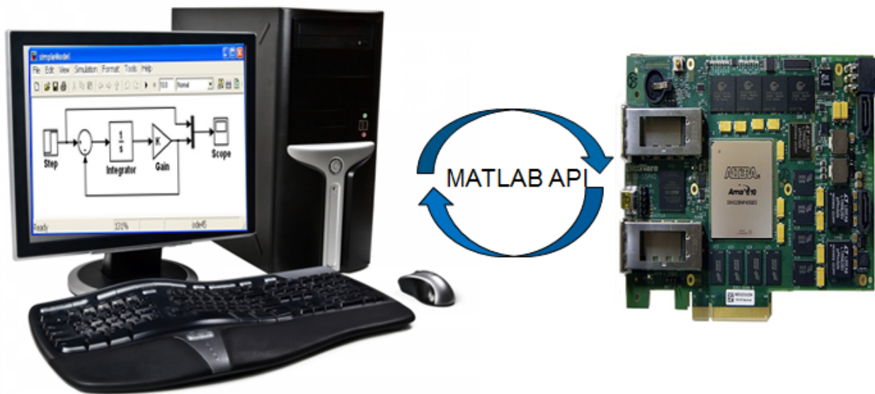
Figure 10-16: Hardware in the Loop Host-Target Setup
