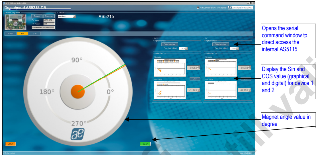
Figure 4: TWI tab, allows access to the AS5215 registers from the serial bus
