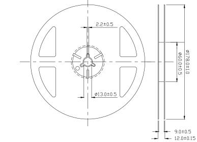
**Note:** The tolerances unless mentioned are ±0.1, unit: mm.
