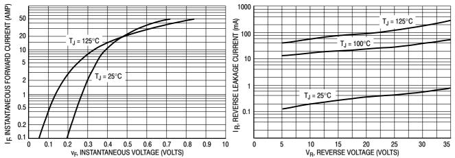
Figure 1. Typical Forward Voltage, Per Leg
