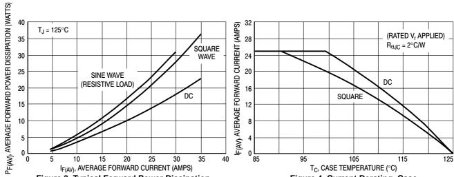
Figure 3. Typical Forward Power Dissipation
