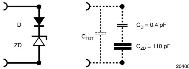
Such a constellation with a Z-diode and a small PN-diode (with low capacitance) in series (anti-serial) is a real unidirectional protection device. The clamping current can only flow in one direction (forward) in the PN-diode. The reverse path is blocked.
