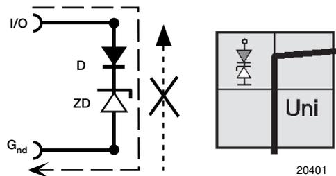
Another PN-diode “opens” the back path so that the protection device becomes bidirectional! Because the clamping voltage levels in forward and reverse directions are different, such a protection device has a **B**idirectional and **A**symmetrical clamping behaviour (**BiAs**) just like a single Z-diode.
