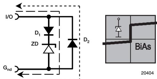
The VBUS054DD-HF4 offers four inputs with such protection circuit inside.
