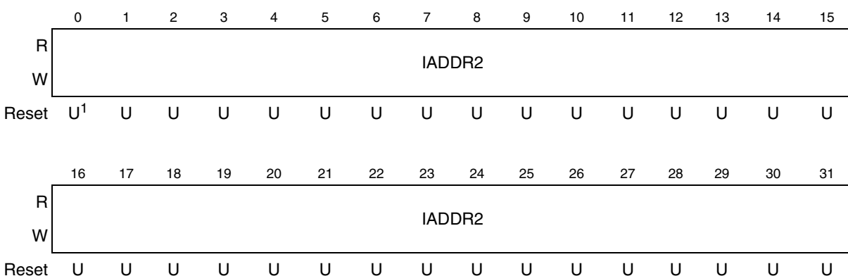
Figure 15-19. Descriptor Individual Lower Address Register (IALR)
