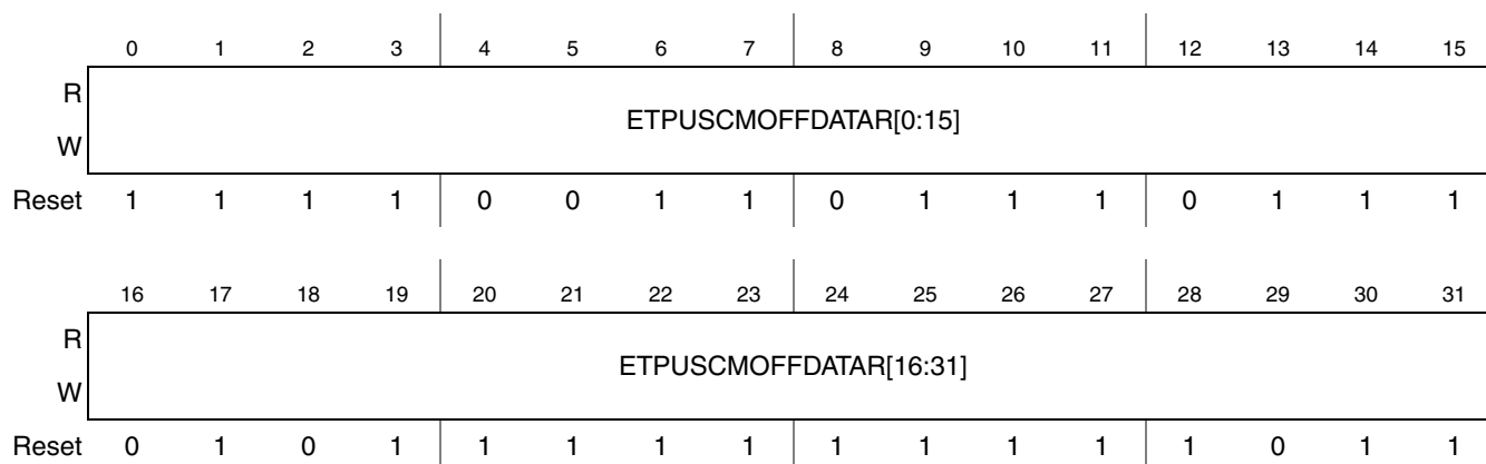
Figure 18-8. eTPU SCM Off-Range Data Register (ETPU_SCMOFFDATAR)
