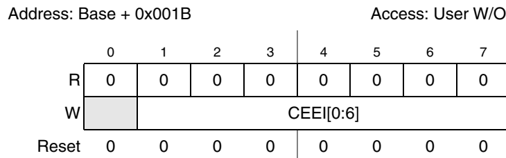
Figure 9-11. eDMA Clear Enable Error Interrupt Register (EDMA_CEEIR)
