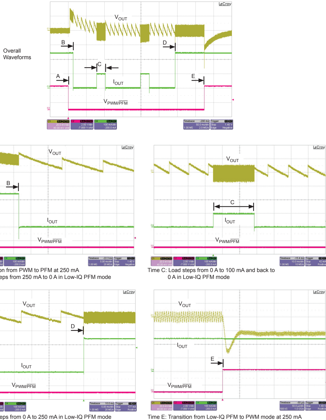
Figure 6: Transitions between PWM Mode and Low-IQ PFM Mode, and Load Transient Responses Using circuit in typical application schematic ( V_{IN} = 12\text{ V} , V_{OUT} = 5\text{ V} , f_{SW} = 425\text{ kHz} )
