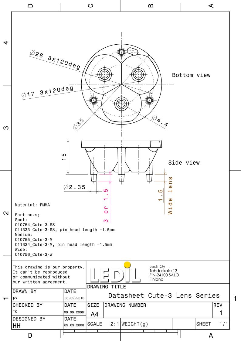
Luminaire: Ledil Oy 10427\_Cute-3-M 10427\_Cute-3-M Lamps: 1 x Cree XR-E 3PCB (white)
