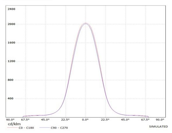
Luminaire: Ledil Oy 10427\_Cute-3-M 10427\_Cute-3-M Lamps: 1 x Cree XR-E 3PCB (white)
