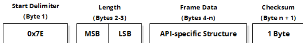
Figure 9: UART data frame structure.
