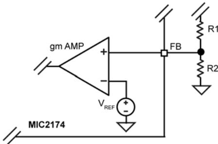
**Figure 8. Voltage-Divider Configuration**
