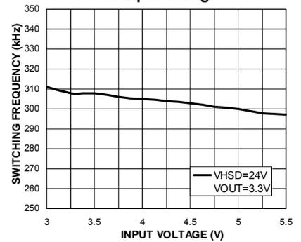
Switching Frequency vs. HSD Voltage
