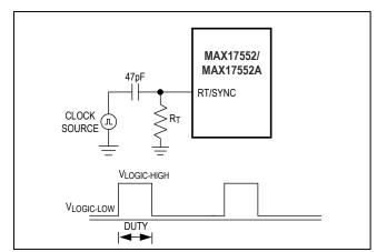
Figure 1. Synchronization to an External Clock
