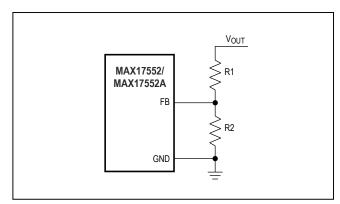
Figure 3. Setting the Output Voltage
