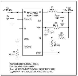
Figure 9. Small Footprint 3.3V, 100mA Regulator
