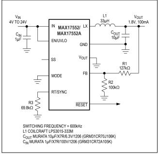
Figure 10. Small Footprint 1.8V, 100mA Regulator
