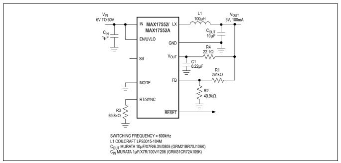
Figure 8. Small Footprint 5V, 100mA Regulator
