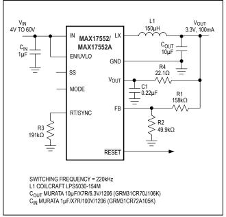
Figure 7. High-Efficiency 3.3V, 100mA Regulator
