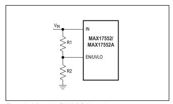
Figure 2. Adjustable EN/UVLO Network
