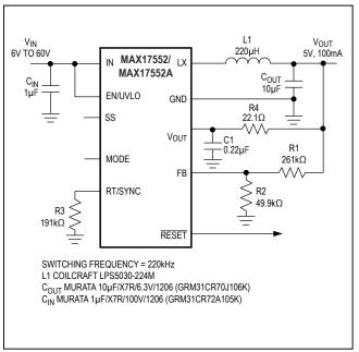
Figure 6. High-Efficiency 5V, 100mA Regulator
