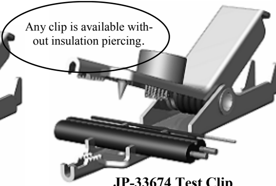
JP-33674 Test Clip Single spike Bed-of-Nails Straight nose 66mm (2.6") long
