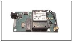
Airborne is a family of fully integrated 802.11 wireless device server and ethernet bridge products designed to provide wireless LAN and Internet connectivity to transportation, medical, warehouse logistics, POS, industrial, military and scientific applications.
