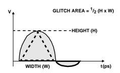
FIGURE 2. OUTPUT SETTLING TIME DIAGRAM
