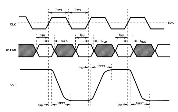
FIGURE 4. PROPAGATION DELAY, SETUP TIME, HOLD TIME AND MINIMUM PULSE WIDTH DIAGRAM
