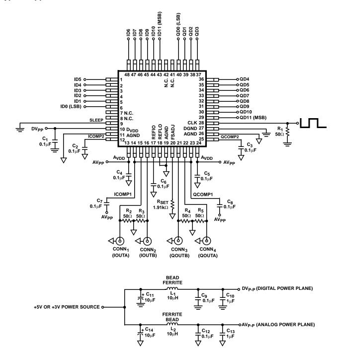
NOTE: Separate analog and digital grounds should be used, in which case the grounds should be tied together at a single point near the device. The analog and digital grounds should be connected together by a thin single trace and never connected together by an inductor.
