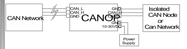
The CAN network must be terminated at both ends according to the CAN specification. Networks not properly terminated may have data errors, or miss the data completely. The CANOP creates two new ends to the CAN network. Space is provided on the board for a termination resistor on each side, R6 and R8. A 120-ohm resistor is recommended for the termination. If the CANOP is not at the end of the network, it should not be terminated.
