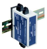
The CAN is connected to the system through terminal blocks. A power supply of 10-30 VDC is required. Model CANOP is housed in a rugged DIN-rail mountable box, making it easy to install in an industrial cabinet.
